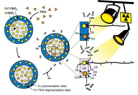
the catalyst particle's shell outer subsequent activation. By pre-contacting catalyst with TEAI, in-situ ethylene oligomerisation sites could be generated. Typically, an olefinic comonomer (i.e., 1-hexene) is added externally to the reaction mixture and has diffuse through the polymer growing catalyst material to arrive at the catalytic sites. We envisioned that it would be advantageous if the co-monomer generated on the TEAI-
